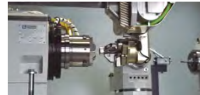
M Motion Gantry integrated in the machine
