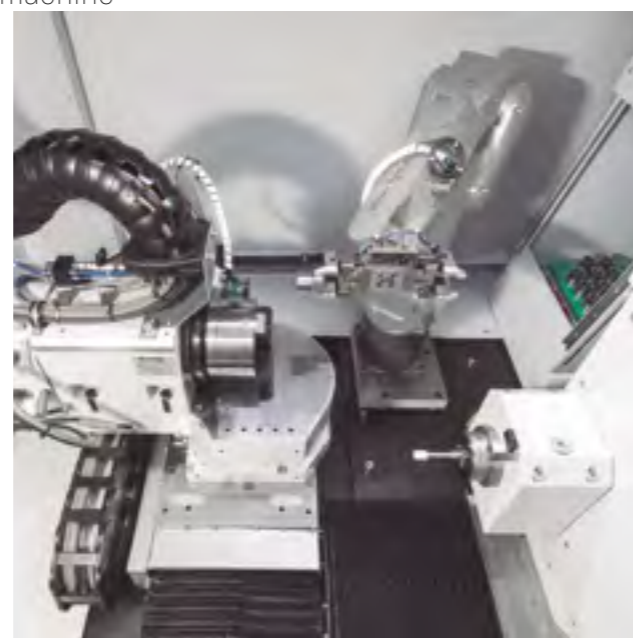
M Flexmotion Robot integrated in a cell coupled to the machine
