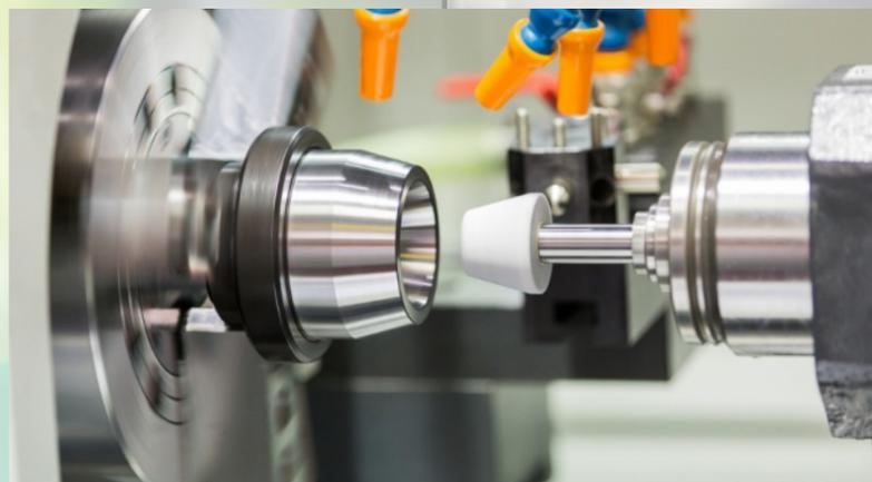
Grinding process of interior cone
