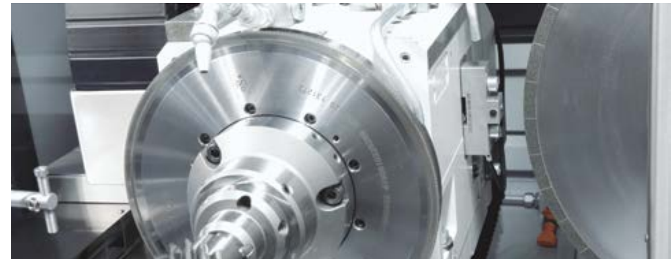
X and Z axes reference block for wheel touch offset reference to avoid manual setting
