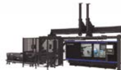
L Hybrid Combination of an external gantry and an external robot cell
