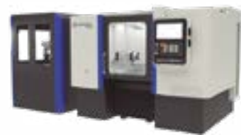
M Flexmotion Robot integrated in a cell coupled to the machine
