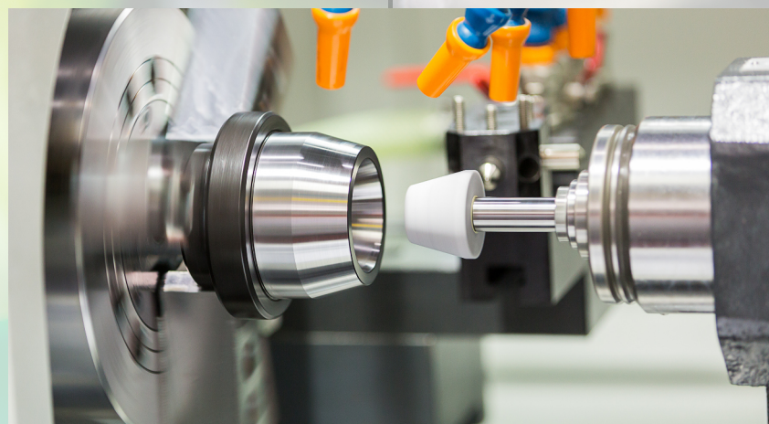
Grinding process of interior cone
