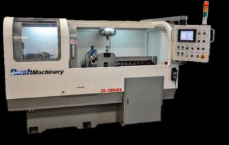
Our machines are for: Truing and dressing Diamond & CBN wheels Cutting off carbide & HSS rods and tools Cutting, Pre-pointing, and chamfering carbide & HSS rods Chamfering carbide & HSS rods Balancing wheels and tools Grinding PCD tools Filtering grinding oil Sharpening drills and tools.
