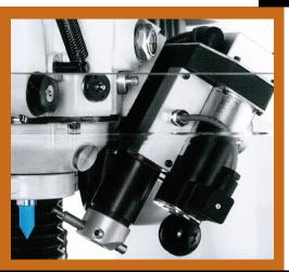
With its special simultaneous 3D abrasive cone movements, the ZSM vertical center hole grinding machine, built by ws technica technology gmbh in Switzerland, produces extremely accurate geometric 60 degree center bores with a roundness of less than 1µm!
