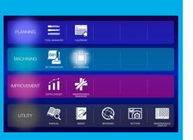
Esoma is specialized in retrofit of HAUSER jig grinding machines with in-house developed jig grinding software and HMI user interface for FANUC controls.
