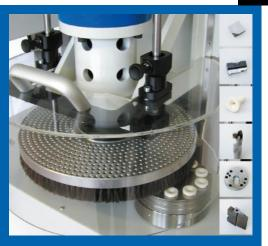
Gerber systems enable the machining of workpieces made of hard materials such as CBN, PCD, Sapphire, Ruby, Ceramic, Carbide, and also Aluminum, Brass and Plastics. Specially developed machines in modular design enable the machining of flat, turned and rotary tools.
