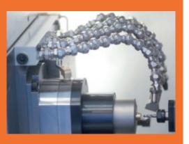
3D printed titanium coolant nozzles from InnoGrind ideally pair with stainless steel coolant lines from HirtLine.
